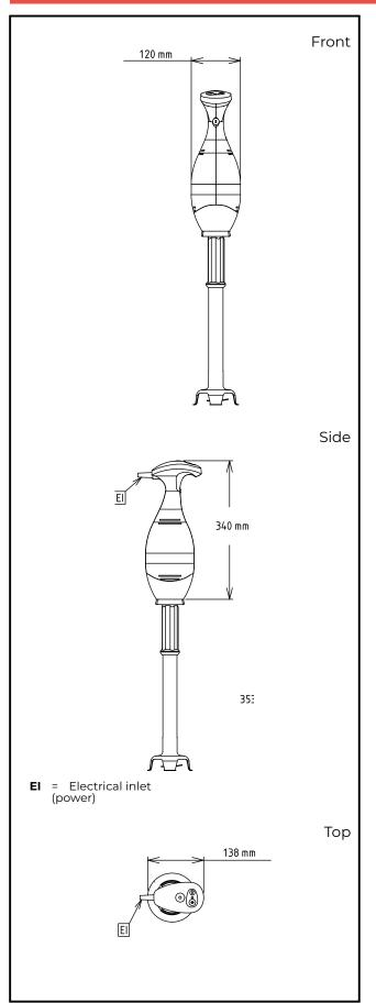
Electric Supply voltage: 220-240 V/1 ph/50/60 Hz Electrical power, max: 0.35 kW 0.35 kW **Total Watts:** Key Information: External dimensions, Width: 138 mm External dimensions, 120 mm Depth: External dimensions, 340 mm Height: **Shipping weight:** 3 kg
